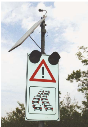
TrafiCam Collect-R installed on existing structures
